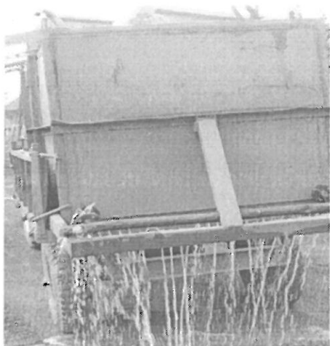
Water sprinkling on roads through mobile water tanker of size – 2.9 m x 1.5 m x 1.3 m
