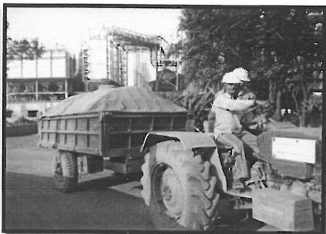
Photo: 12- Flue dust collected covered with tarpaulin and used for briquette making
