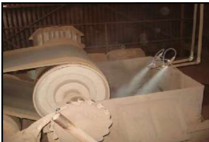
Photo:4- Dry Fog dust suppression system at screen house, underground bunker & conveyors
